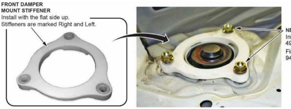
NEW NUTS (3) Initial torque: 49 N·m (36 lb-ft) Final torque: 94 N·m (69 lb-ft)
