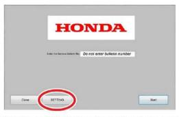
Update the PGM-FI or A/T software by selecting the i-HDS Diagnostic System icon. Refer to Service Bulletin 01-026, Updating Control Units/ Modules.
