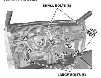
7. Remove the dashboard, then remove the harness clip.
