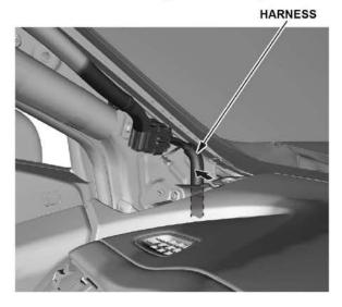
2. Remove the harness clips from the gauge control module.
