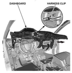
8. Remove the dashboard wiring harness.
