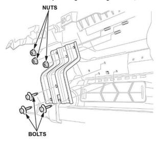
11. Install the dashboard, and torque the large bolts to 17 N·m (13 lb-ft) and the small bolts to 8 N·m (5.9 lb-ft). Then install all other parts in the reverse order of removal.
