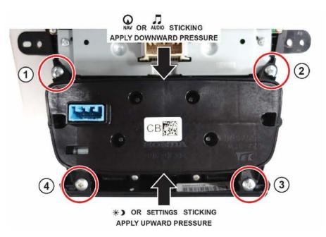
6. While applying upward or downward pressure, tighten the screw behind the sticking button first, then tighten the other three screws while continuing to apply pressure.
