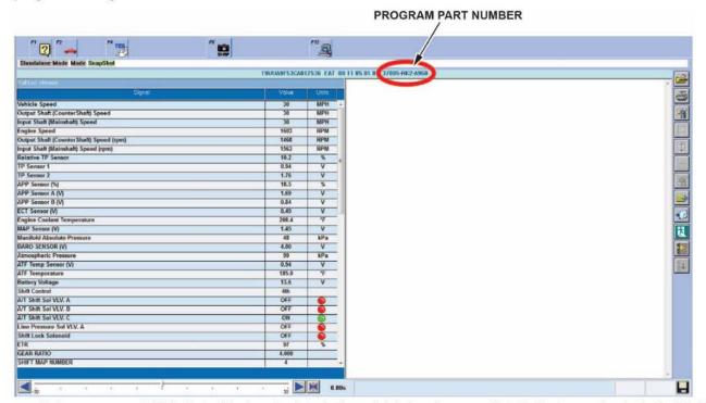
• If the program P/N is listed below (or later), the vehicle has been updated. Go to service bulletin 17-007, 2012–13 ZDX: Judder from the Torque Converter Lock-Up Clutch After Software Update.
