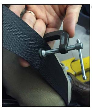
Squeeze the button using a small "C" clamp (approximately 1.5-inch span) to complete the installation.
