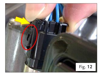
➤ Detach the connector from the sensor while keeping the retainer clip pressed (1) - Fig. 13.
