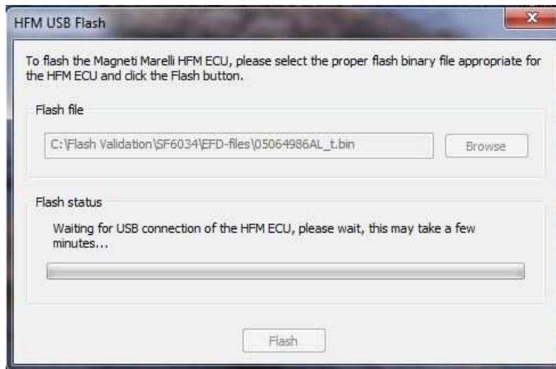
Fig. 14 HFM Status Pop-up (While waiting for connection)
