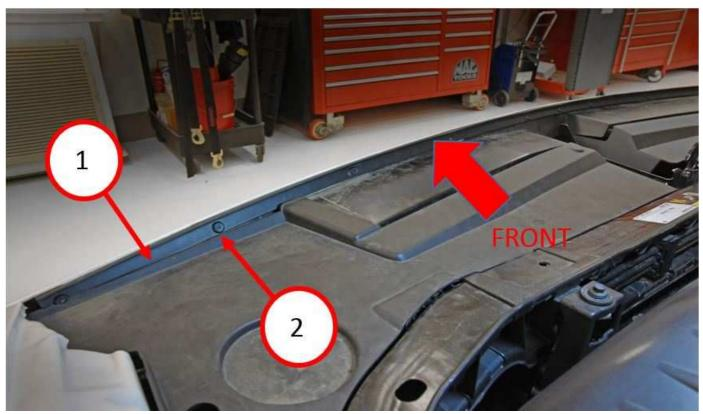
Fig. 2 View of Hood Seal and Retainers (shown with upper close out panels in place)
