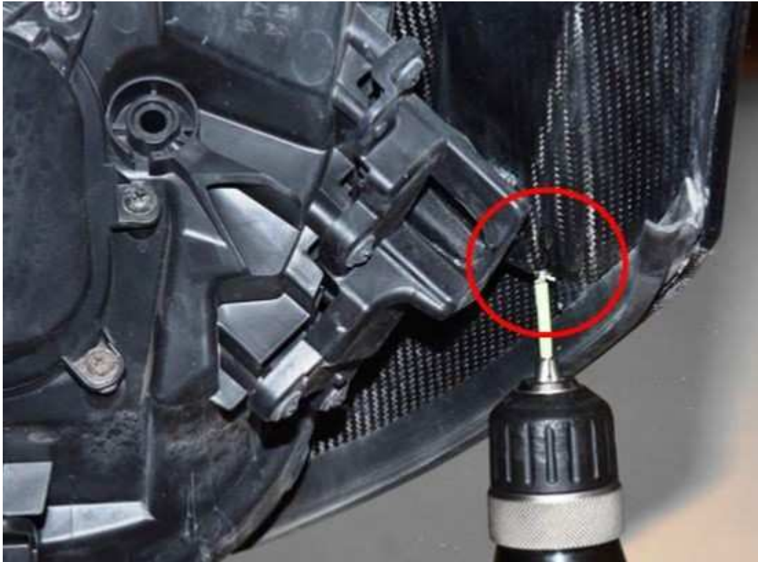
Fig. 3 Drilled Drain Hole
