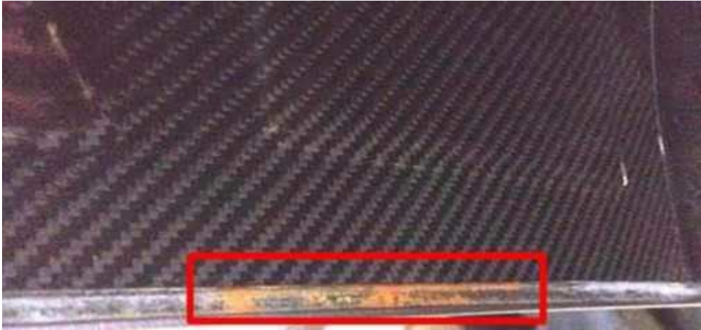
Fig. 6 Hood Liner Seam Corrosion
