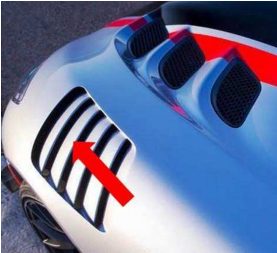
Fig. 5 Direction To Water Flush Hood
