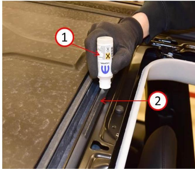
**Fig. 11 Weather Strip Lubricant**
