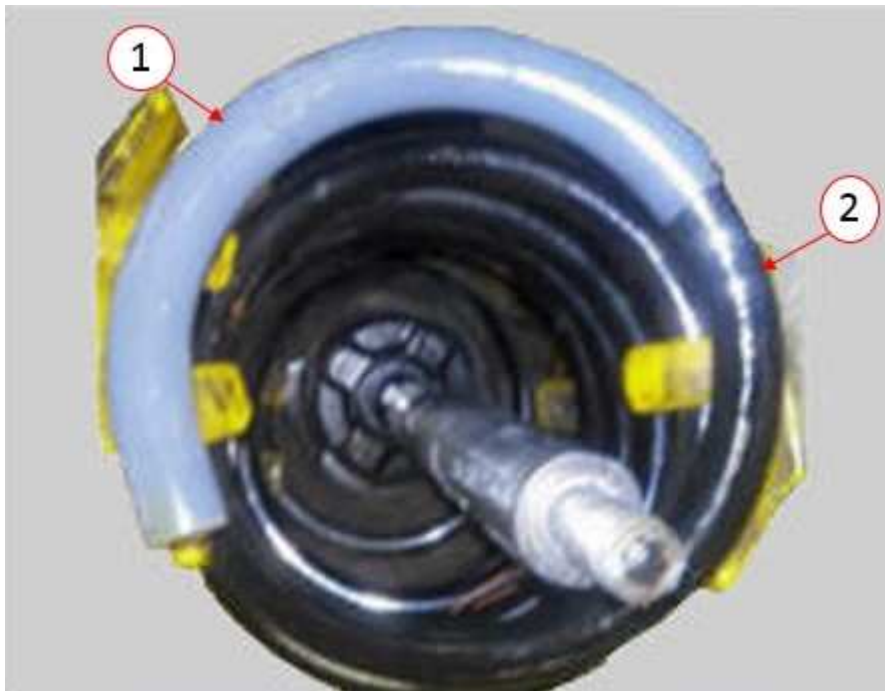
Fig. 1 Sleeve Position on Front Coil Spring
