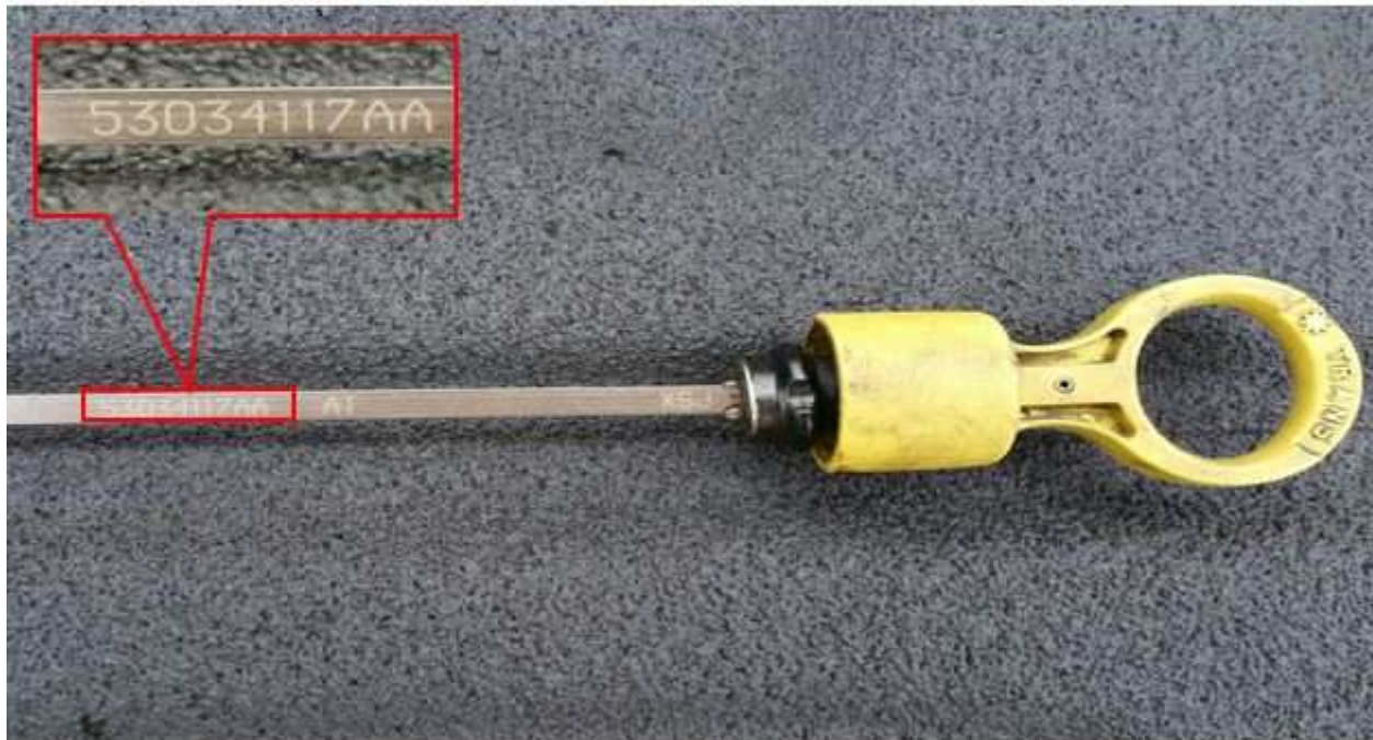
Fig. 1 Location Of Part Number On Oil level Indicator
