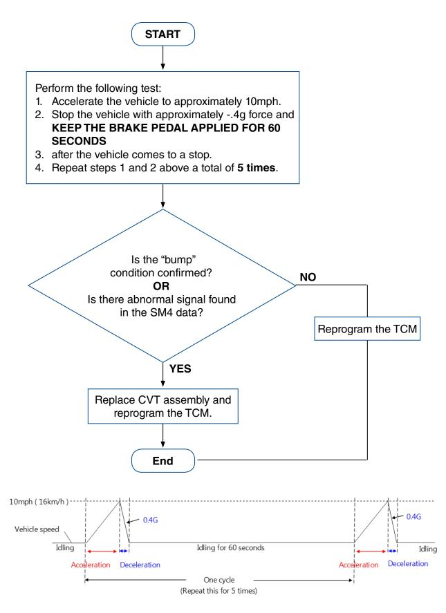
• While performing the testing above, determine if the "bump" condition can be confirmed and / or if the data graph shows any chain slippage. Examples of "OK" and "NG" graphs are supplied below for reference to help make a proper determination.
