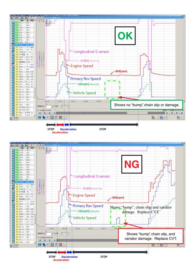
• If the bump condition is confirmed, there is most likely variator damage requiring CVT assembly replacement. Follow the service procedure in the applicable Service Manual when replacing the CVT assembly is required.
