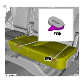
Make sure the 2 clips are correctly latched.
