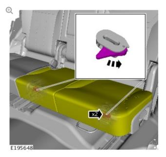
Release the 2 clips retaining the second row left seat cushion.
