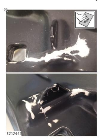
Using the sandpaper in the repair kit prepare the microcracks for the filler.
