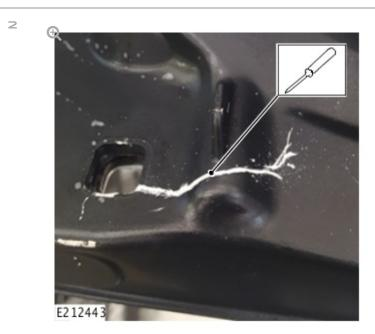
Using a suitable flat blade screwdriver, open up the microcrack so the filler can be applied.
