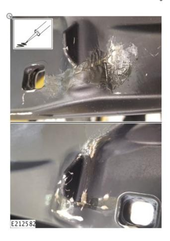
Mix the TEROSON PU 9225 filler from the repair kit and apply to the microcracks as shown.
