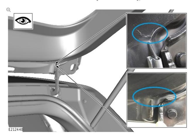
Typical location of the microcracking (can occur on either or both sides of the tailgate).
