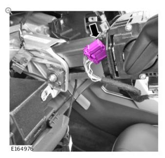
Remove the electrical connector C2LS41 (Green) from the module steering wheel.
