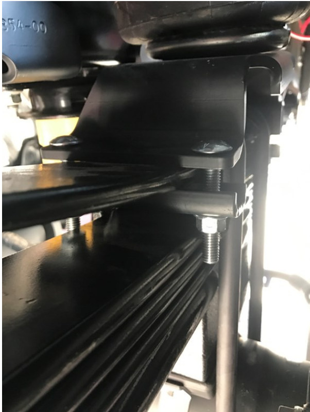
Figure 3. Lower clamp affixed directly to overload leaf spring
