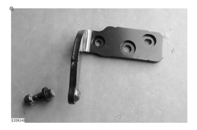
Example: damage to the deployable luggage compartment floor operating arm.
