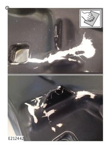
Using the sandpaper in the repair kit prepare the microcracks for the filler.
