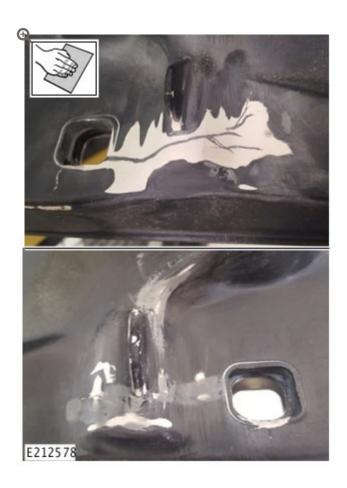
Using the P400 sandpaper from the repair kit, flatten the filler.
