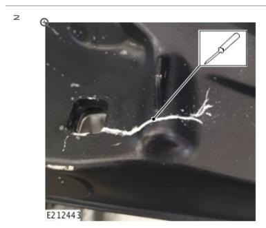
Using a suitable flat blade screwdriver, open up the microcrack so the filler can be applied.
