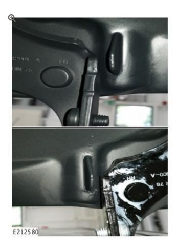
Paint the repaired area with the EQUILIBRIUM spray paint from the repair kit.
