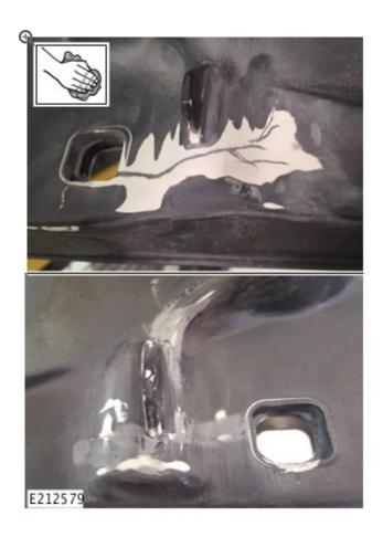
Clean the surface using the surface cleaner wipes from the repair kit.
