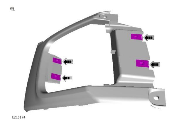
Install 4 new retaining nuts onto the rear bumper finisher.
