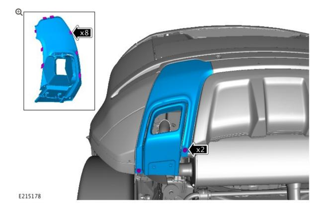
Remove the 2 fasteners from the rear bumper finisher.
