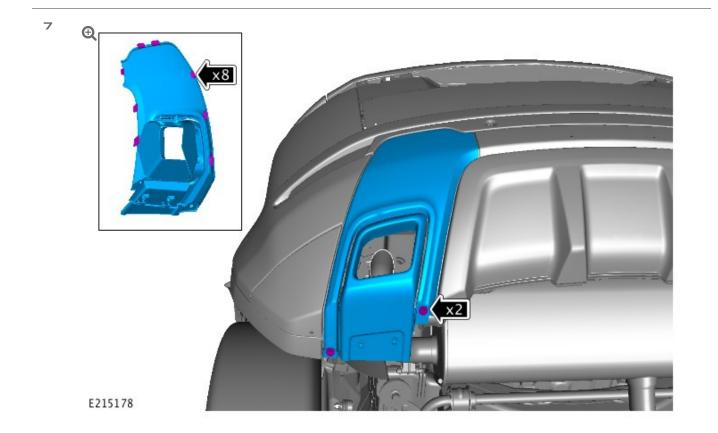
Install the rear bumper finisher and exhaust finisher.
