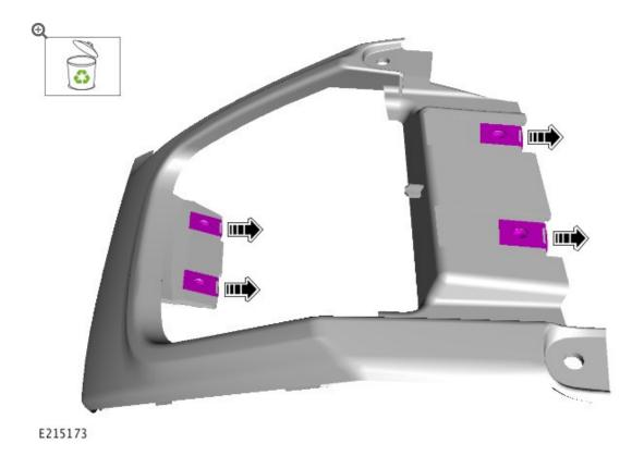
Remove the 4 retaining nuts from the rear bumper finisher.
