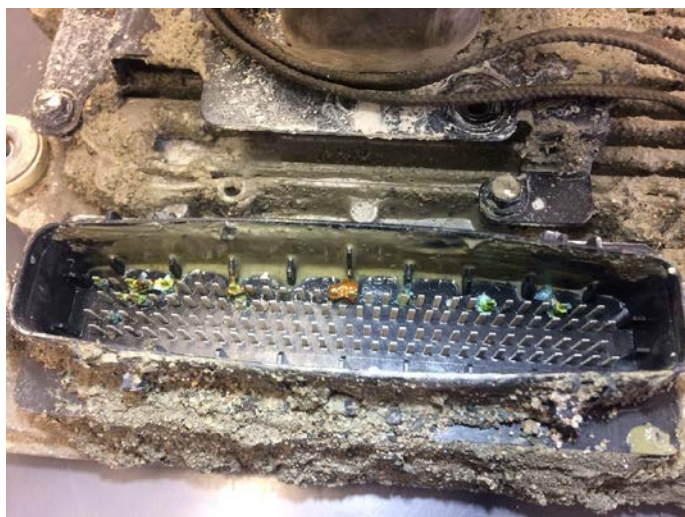
Figure 9 – ACM 21-pin and 120-pin Connector Inspection
