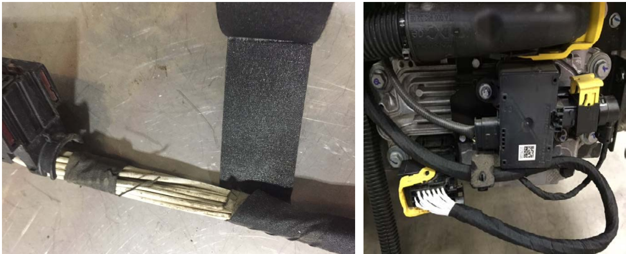
Figure 11 – Anti-Chaffing Tape Installation
