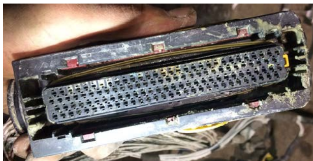
Figure 8 – ATS Harness 21-pin and 120-pin Connector Inspection
