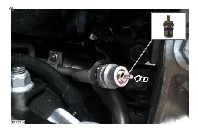
Use a suitable tool to install new A/C system charge port Schrader valves (turn clockwise).
