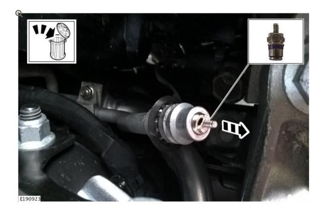
Use a suitable tool to remove and discard the A/C system charge port Schrader valve (turn anticlockwise).
