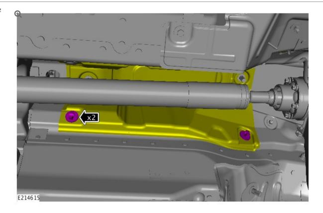
Remove and discard the 2 transmission tunnel Noise, Vibration and Harshness (NVH) material clips.
