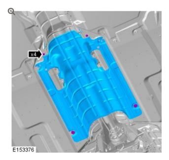
Install the exhaust heatshield.
