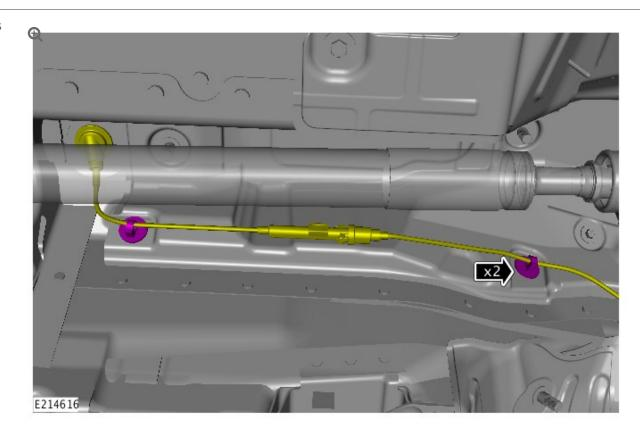
Install the lower EPR cable into the 2 clips.
