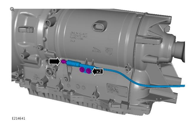
Install the new lower EPR cable.
