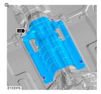
Remove the exhaust heatshield.
