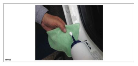
4. Remove the paste completely by polishing.
