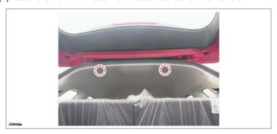
3. Partially peel back the rear part of the headliner from the seaming welt.
