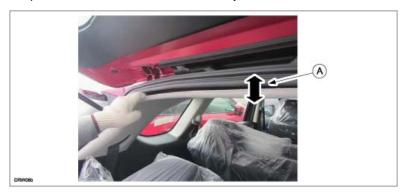
4. Tighten the four (4) liftgate hinge nuts (A) on the body side. There are two (2) nuts per side.
