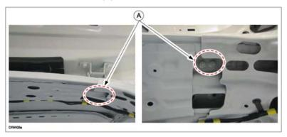
NOTE: Recommended socket: 14mm. 30mm (length) so that its easier to fit into the tight/narrow space.
