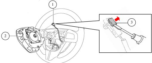
Two types of old and new stopper plates exist. The exact switching date from the old to new stopper plate is unknown. Please first confirm the configuration of the stopper plate used on the vehicle in repair, and then use the one with the same configuration.
