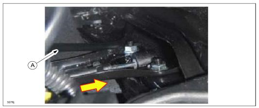
14. Press the cable firmly in by hand and secure it along the bracket (as shown below).
