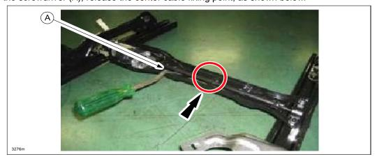
**CAUTION:** After removing the cable, DO NOT operate the slide switch, otherwise, it may cause damage to the adjuster unit.
