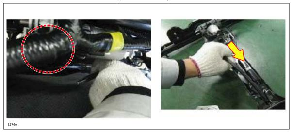
11. Pull the cable in the direction of the arrow (as shown below) to remove it from the gear box.
