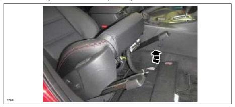
7. Insert a screwdriver between the frame and the cable (shown in the red rectangle below).
