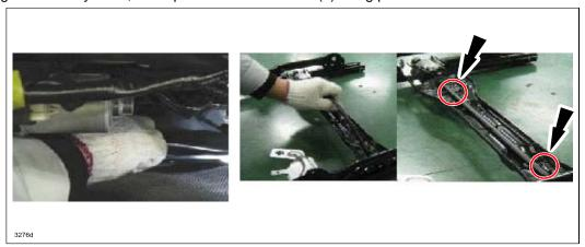
**CAUTION:** When removing the cable, remove it from the motor side first. If it is removed from the gear box side first, the engagement position could be misaligned.
