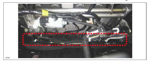
16. Check the installation of the cable to the motor and to the gear box (A) and the installation of the cable along the frame (B).
