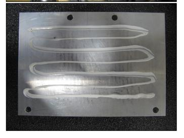
37. Mount motor controller 20 onto electrical mounting bracket (with heat sink, for 6.5kW motor-equipped vehicles) as shown and install the main motor controller wiring connector.
