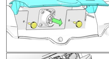
3. Keeping the hood parallel with the ground, Pull the hood forward to release it from the grommets. Carefully lift the hood away from the vehicle.
