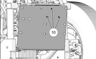
14. Remove zip ties from the electrical mounting bracket, and from the vehicle's sub-frame as shown.
