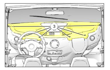
II. Lift upper dash to access and disconnect electrical connectors. Remove dash from vehicle.
