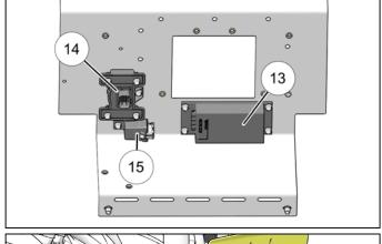
24. Install new mounting bracket onto vehicle, and loosely install two lower mounting screws on new electrical mounting bracket. Leave bracket tilted for access.
