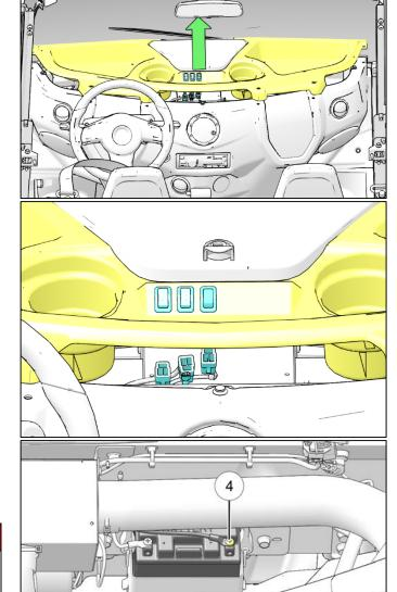
III. Disconnect negative (-) battery cable ④ from the auxiliary battery under the dash.
