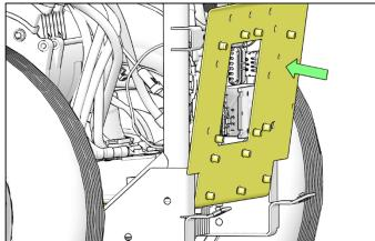
25. Install contactor (16) into new location. Torque bolts to specification.
