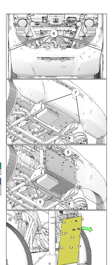
12. Remove bolt from left side of charger mounting bracket, install horn and reinstall mounting bolt.
