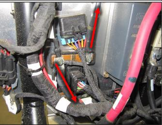
33. Install new connector routing clip onto 48V fuse block and install it into the electrical mounting bracket above the BMC.
