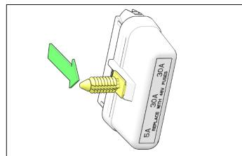
34. Install new connector routing clip into service disconnect. Install service disconnect into new mounting location next to the left frame tube.
