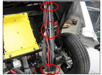
47. Using zip-ties supplied in the kit, retain the bulk of the main harness against the sub frame as shown.
