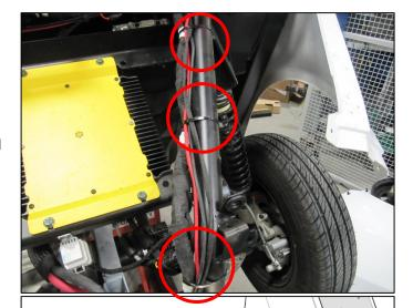
15. Remove two contactor mounting bolts and remove contactor from electrical mounting bracket.
