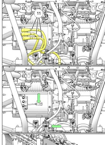
21. Disconnect motor temperature sensor and motor speed sensor.
