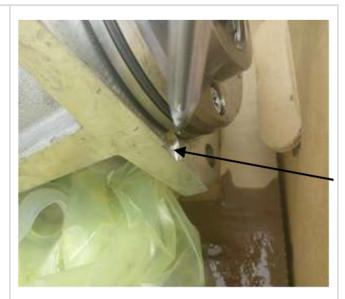
The fuel lip seal in the high pressure pump can fail when low side fuel pressures are extremely high. High fuel pressure is caused from a restriction on the return side of the fuel system. Visually inspect the OEM return fuel lines from the fuel filter module back to the tanks. Look for any severe bends or kinks in the line. The photo to the right shows where the return fuel line was kinked when it was connected to a fuel cooler. Make any repairs needed.
