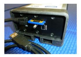
After loading the appropriate config file to the SD card, insert it in the DiCE.
