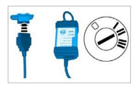
Plug the DiCE unit into the vehicle's diagnostic connector and turn on the ignition or start the engine
