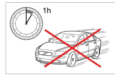
Caution! After installing the component, wait for a minimum of 1 hour before driving the vehicle.
