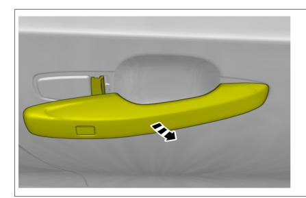
Lift the marked component forward.
