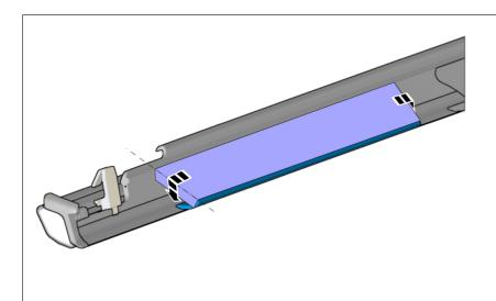
Note! Make sure that the tape has not detached from the edges of the component.
