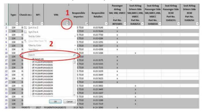
3. The column marked with an X indicates which airbag/s to replace.
