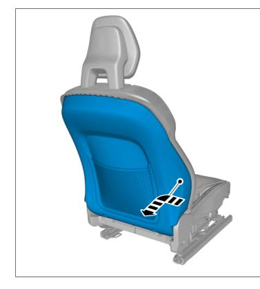
On both sides. Remove the marked part.
