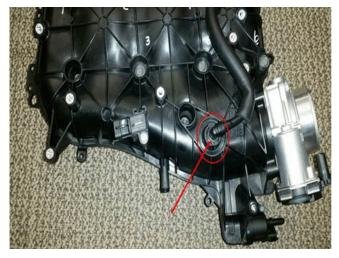
If you encounter a vehicle with the above concern, check for leak at the foul PCV tube to manifold connection as illustrated above.
