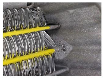
This condition may be the result of excessive thermocycles within the cooling system caused by excessive cycling of the thermostat. These excessive thermocycles within the coolant system may cause the tubes to fatigue, crack and leak at the radiator headers. To correct this condition, new thermostat has been designed that eliminates the thermostats excessive cycling.
