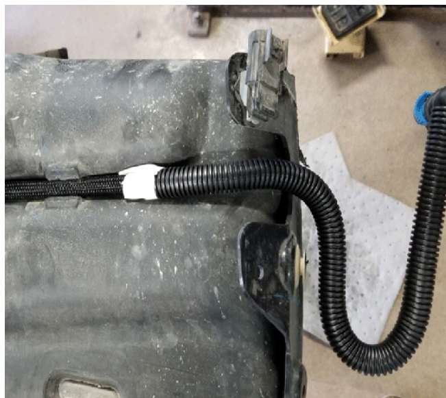
Original design fuel feed line at tank
