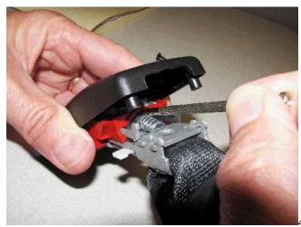
Insert a small screwdriver, or similar tool, between the spring and the red release button cavity.
