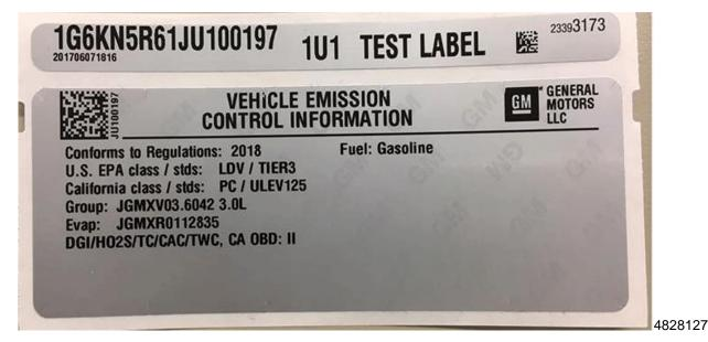
**Important:** The new label will come with a small "waste strip" at the top that contains the entire VIN of the vehicle. Do NOT install the "waste strip" onto the vehicle. It is used for identification purposes ONLY.
