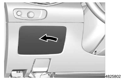
1. Remove instrument panel fuse block cover.
