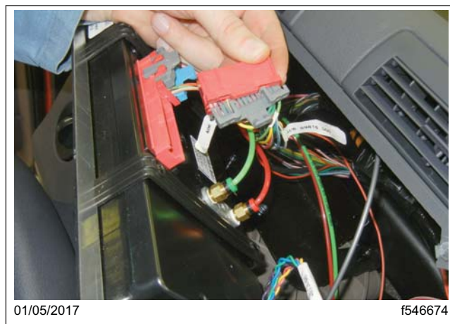
Fig. 14, ICU 2A connector Terminal Locks
