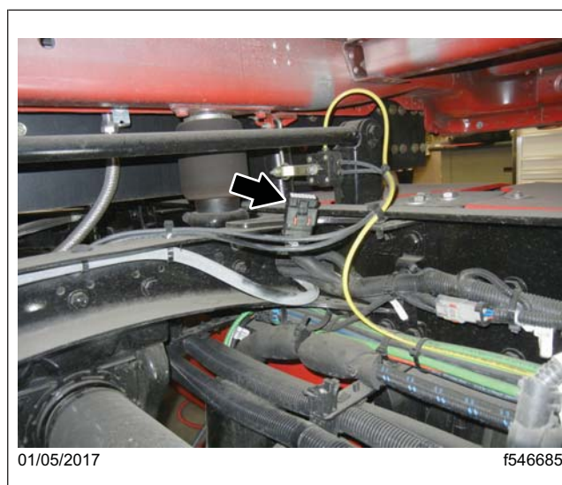
Fig. 27, CPDM Harness Capped
