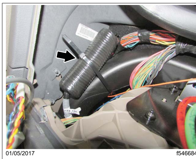
Fig. 24, PLC Bundle Mounting
