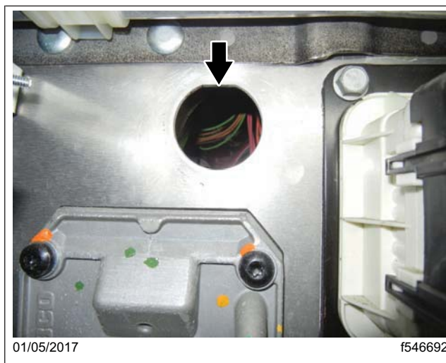
Fig. 32, Bulkhead Connector 1A Cavity on the Frontwall
