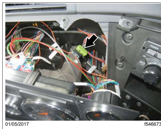
Fig. 13, Splice Pack Routing
