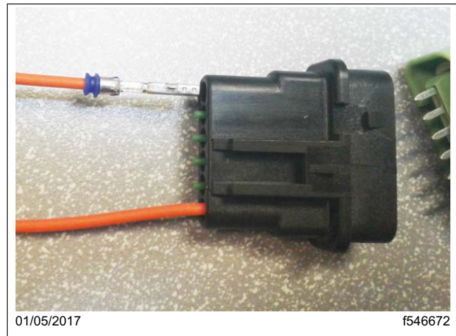
Fig. 12, Splice Pack Terminal Insertion
