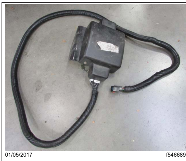
Fig. 29, CPDM Removed from the Vehicle
