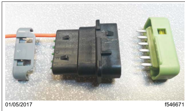
Fig. 11, Splice Pack Cover and Lock (removed)
