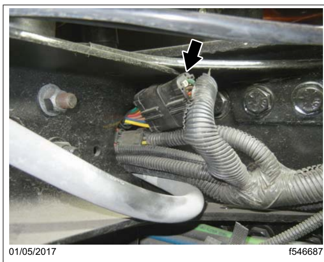
Fig. 25, CPDM Harness Connector
