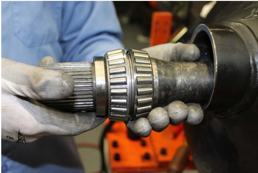
Figure 9 – Thru-shaft and Bearing Assembly Installation
