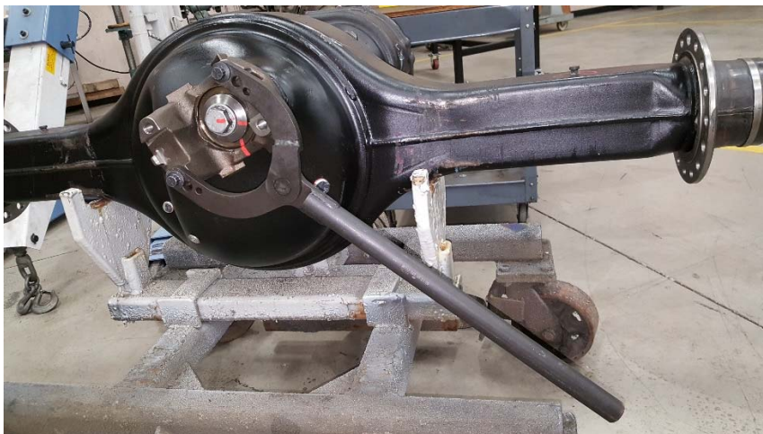
Figure 3 – Output Yoke Bolt and Washer Removal
