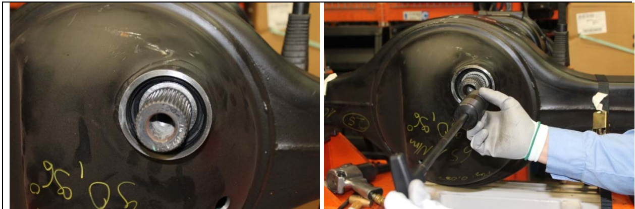
Figure 5 – Thru-shaft Oil Seal Removal
