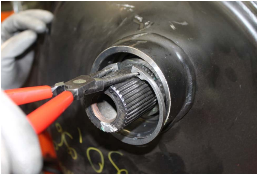
Figure 6 – Snap Ring Removal
