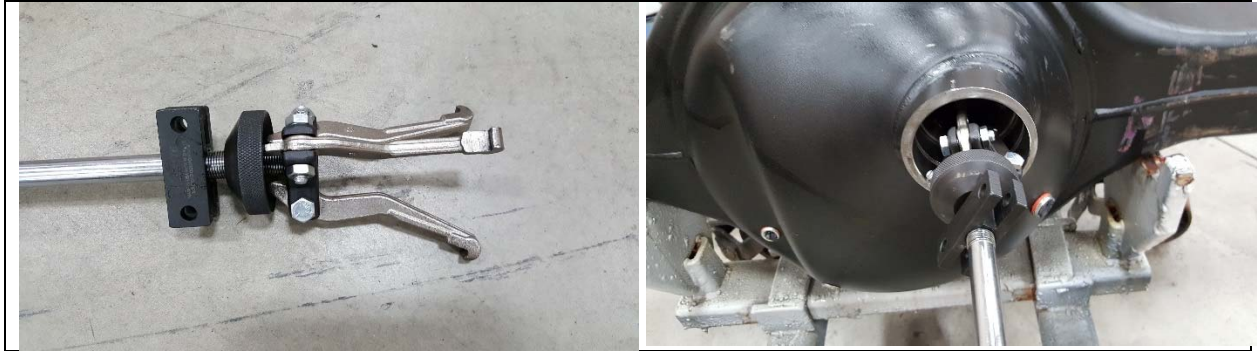
Figure 8 – Bearing Race Removal
