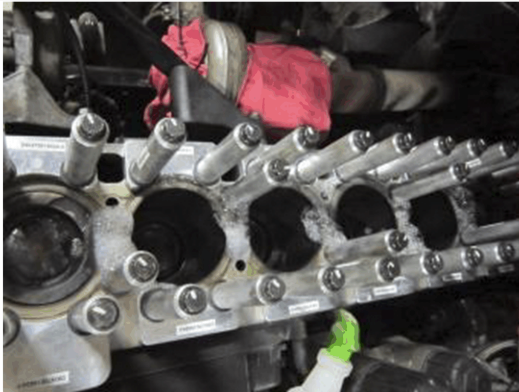
Example A - Multiple Upper Liner Seals Leaking
