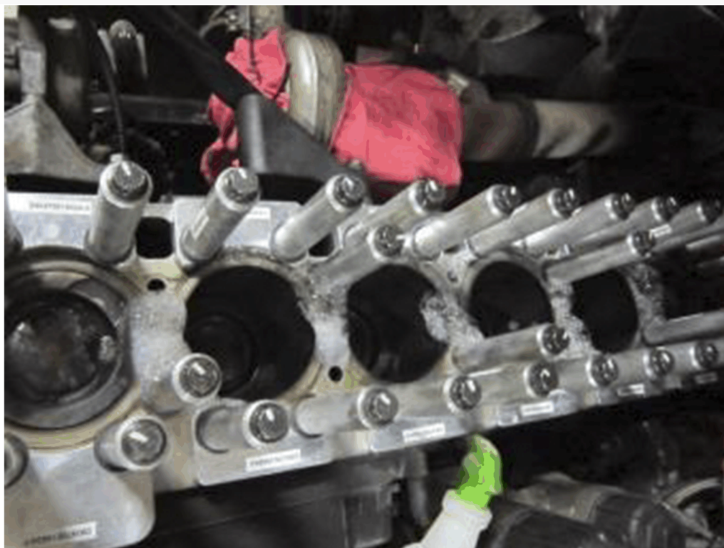
Example A - Multiple Upper Liner Seals Leaking
