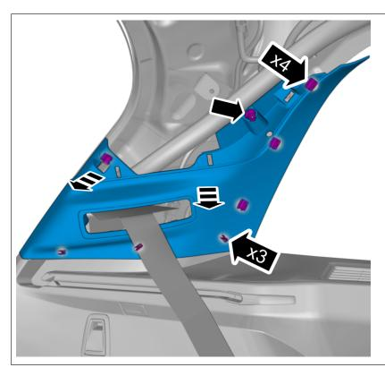
Right-hand side Remove the nut. Remove the marked part.
