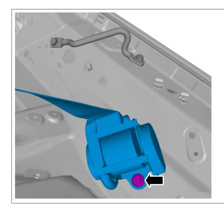
Right-hand side Remove the screw. Remove the marked part.
