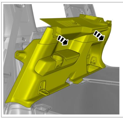
Right-hand side Fold marked part to one side.
