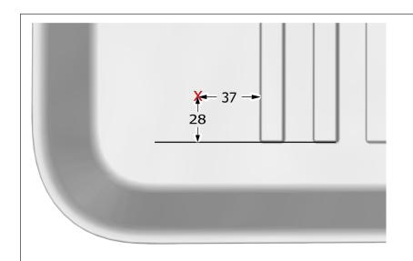
Left-hand side Mark using a pen Measure and mark as illustrated.
