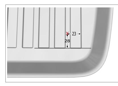
Right-hand side Mark using a pen Measure and mark as illustrated.
