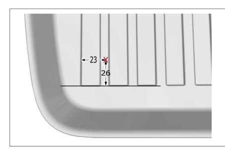
Left-hand side Mark using a pen Measure and mark as illustrated.
