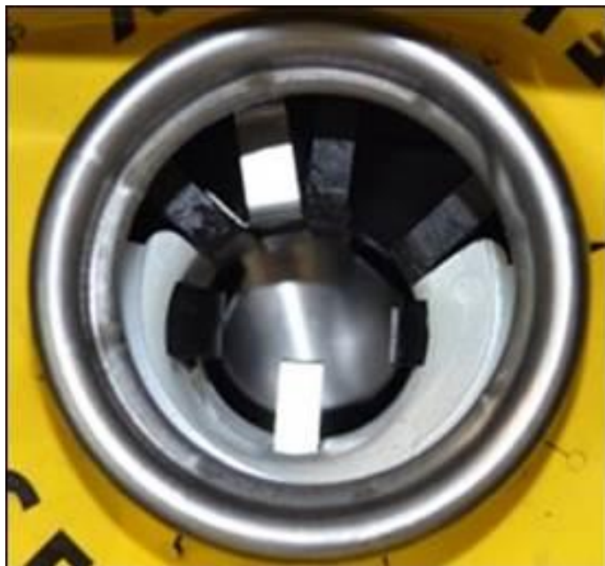
Figure 1. Misfueling guard installed in the filler neck.
