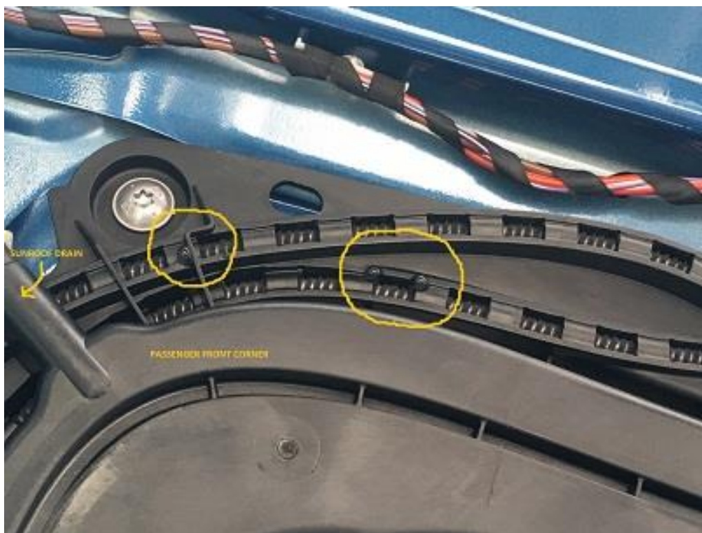
Figure 2: water leaking through sunroof cable guides
