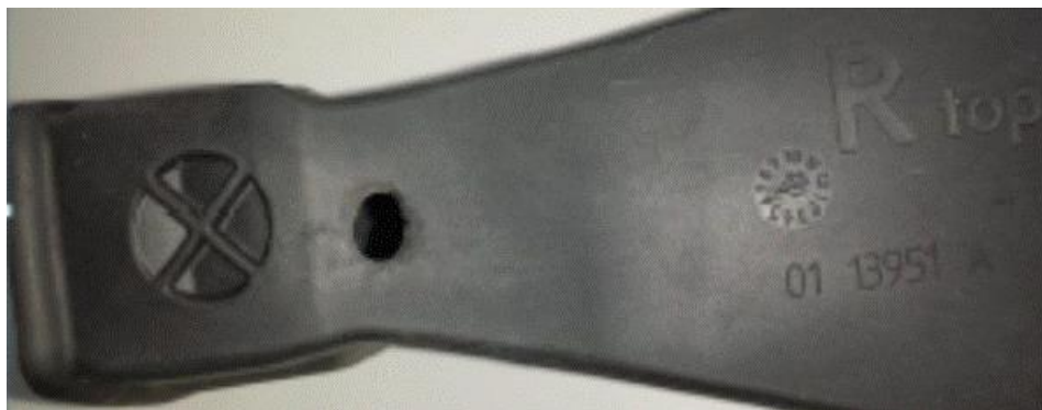
Figure 3. Example of door arrester cover with water drain hole for left side of the vehicle ("R top")
